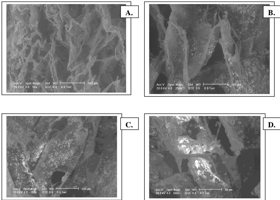
**Fig. 2.** SEM images of COL sponge (A) and COL- $\beta$ -TCP biocomposites (B, C, D).
