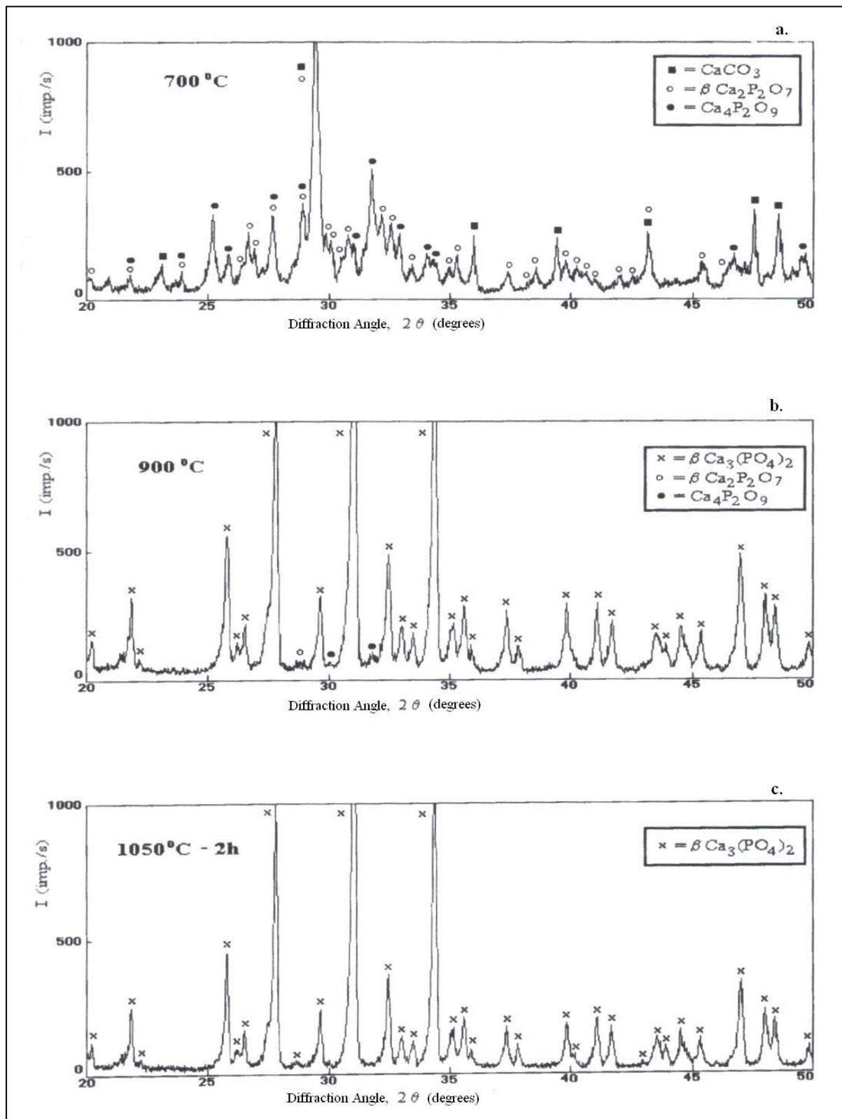
**Fig. 1.** Kinetics of TCP formation analyzed by X-ray diffraction.
