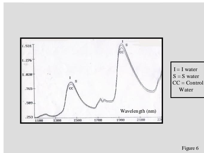
**Figure 6.** Infrared reflectivity spectrum of one emulsion. Reflectivity (R) was measured for one emulsion prepared with three types of water, and  $\log(1/R)$  is plotted *versus* wavelength. I: emulsion in I water, S: emulsion in S water, CC: emulsion in distilled water.
