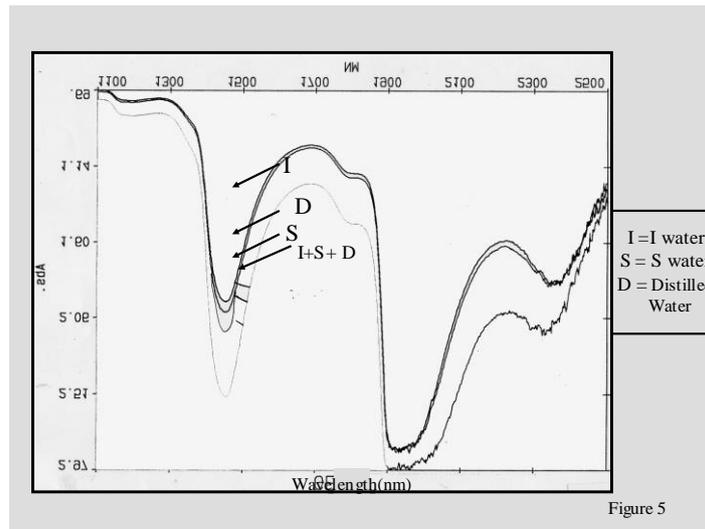
**Figure 5.** Infrared spectrum of water-carbopol gels. IR absorption spectra. The arrows point to the spectra of gels prepared with distilled water (D), I-water (I) S-water (S) and a combination of equal amounts of the three (I+S+D).
