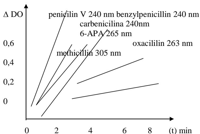
**Figure 2.** The dependence of  $\Delta OD$  on time during the hydrolysis of several penicillins by  $\beta$ -lactamase at pH=7,30 °C, 1 cm optical path. Benzylpenicillin 0.5mg/ml;  $\beta$ -lactamase 12 units/ml; carbenicillin 1 mg/ml, 61 units/ml; penicillin V 1 mg/ml, 24 units/ml; 6-APA 10 mg/ml, 3000 units/ml; methycillin 3 mg/ml, 610 units/ml; oxacillin 10 mg/ml, 1400 units/ml, 0.2 cm optical path.
