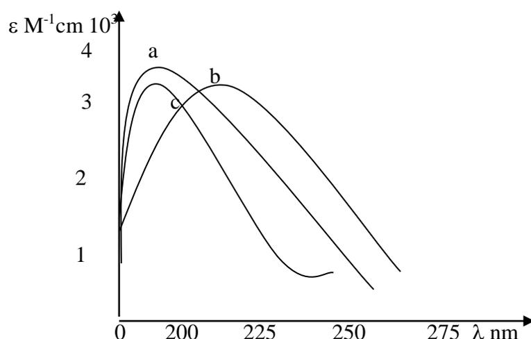
**Figure 1.** Ultraviolet absorption spectra of 6-APA solution in 0.1 M phosphate, pH=7, before (a line) and after (b line) enzymatic hydrolysis. The third curve c which refers to the right-hand side ordinate is the differential absorption spectrum of 6-APA and its hydrolysis product.
