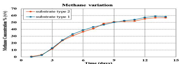
Figure 2. Variation of methane concentration % (v/v) during 14 days of experiment
