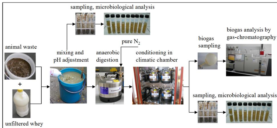
**Fig. 1.** Experimental set-up diagram for the anaerobic digestion experiments
