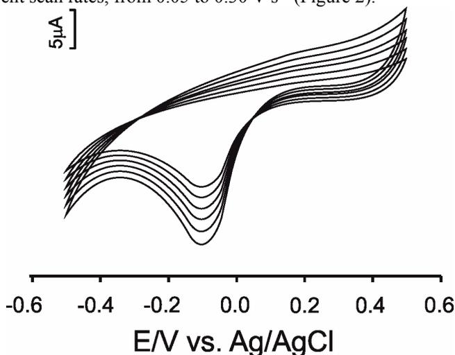
**Figure 2.** Cyclic voltammograms of Ty/CoPc-CPE biosensor registered at different scan rates in  $10^{-4}\text{M}$  serotonin solution (0.01M PBS pH 7.0)
