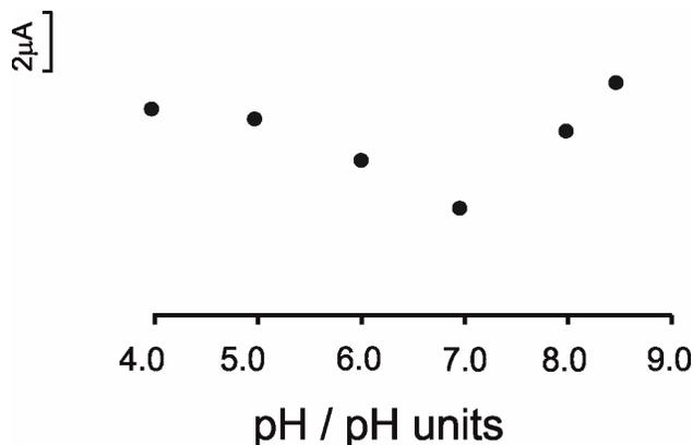
**Figure 4.** The effect of pH value in biosensor response. Conditions: 0.01 M PBS containing  $10^{-4}$  M serotonin. Applied potential: -0.1 V.
