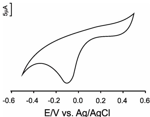
**Figure 1:** Cyclic voltammogram of biosensor in  $10^{-4}$ M serotonin solution (0.01M PBS pH 7.0)
