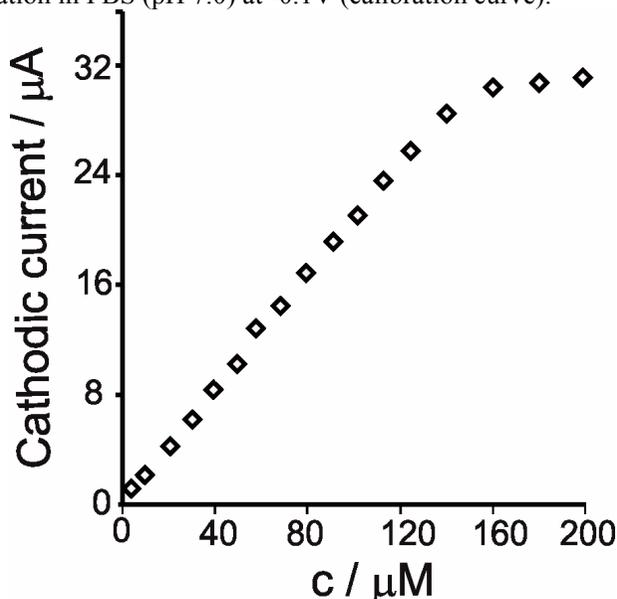
**Figure 6.** The calibration curve between the reduction current and the concentration of serotonin in PBS (pH 7.0) at -0.1 V.
