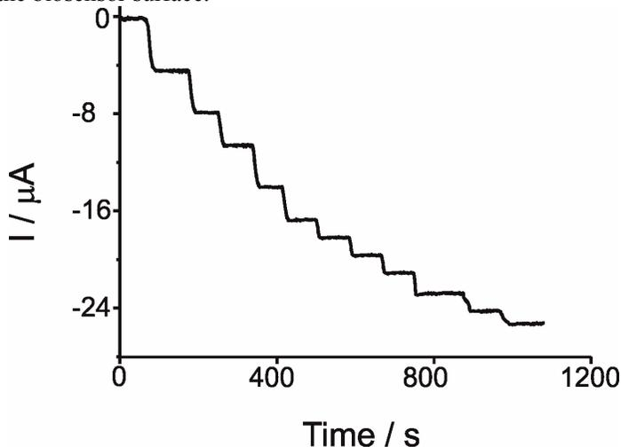
**Figure 5.** Amperometric response of biosensor to serotonin in 0.01 M PBS solution (pH 7.0). Applied potential -0.1 V.
