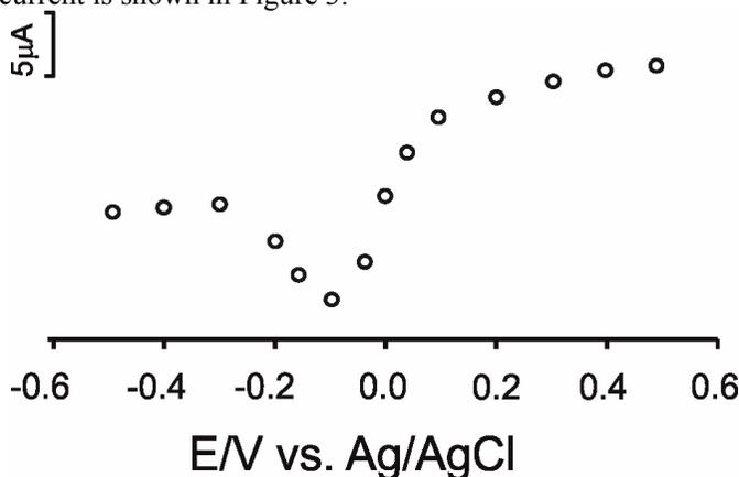
**Figure 3.** Cathodic current-applied potential dependence in 0.01 M PBS (pH 7.0) and  $10^{-4}$  M serotonin under constant stirring.
