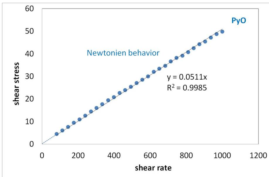
**Figure 7.** Investigation of the Newtonian behavior of pure PyO as protic ionic liquid.
