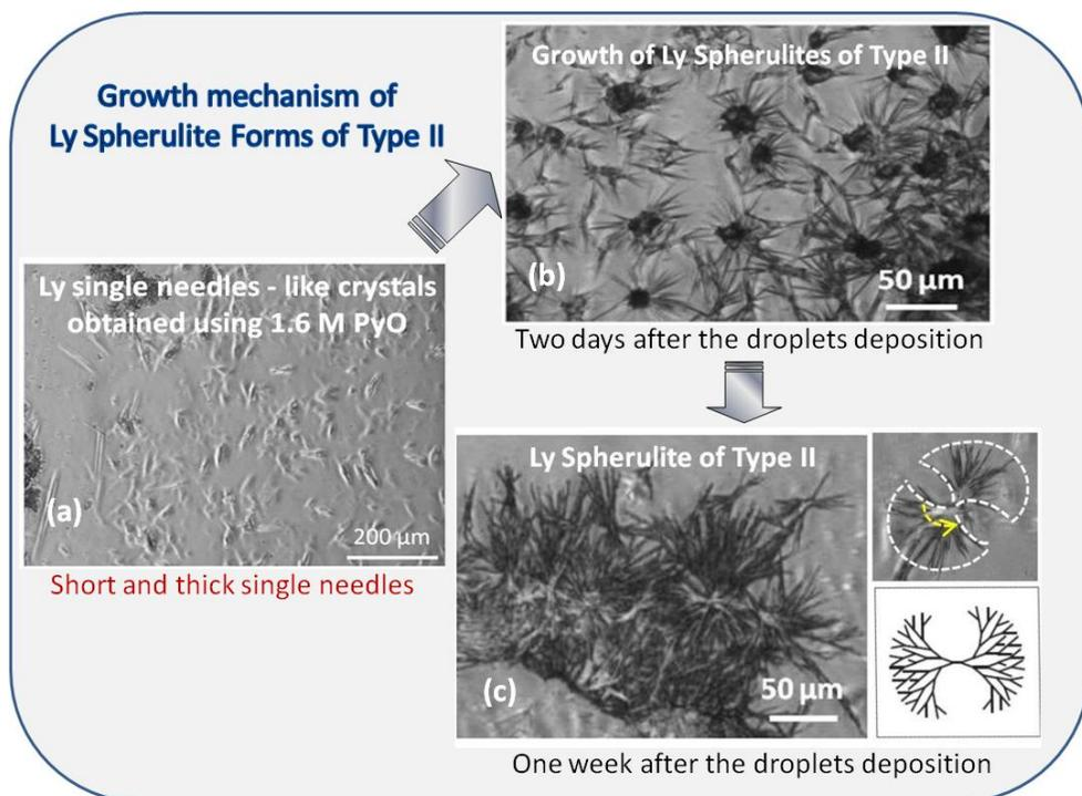
**Figure 4.** Growth mechanism of Ly spherulites using 1.6 M PyO as protic ionic liquid agent in 0.1 M TRIS/crystallant agent.
