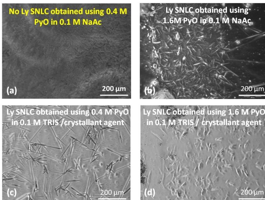
**Figure 2.** Optical images of the initial Ly morphology formed one day after the droplets deposition, using: (a) 0.4 M PyO in 0.1 M NaAc; (b) 1.6 M PyO in 0.1 M NaAc; (c) 0.4 M PyO in 0.1 M TRIS/crystallant agent; (d) 1.6 M PyO in 0.1 M TRIS/crystallant agent.
