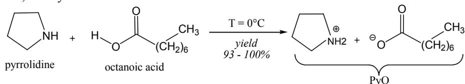
**Scheme 1:** The synthesis of PyO by neutralization reaction of pyrrolidine with octanoic acid
