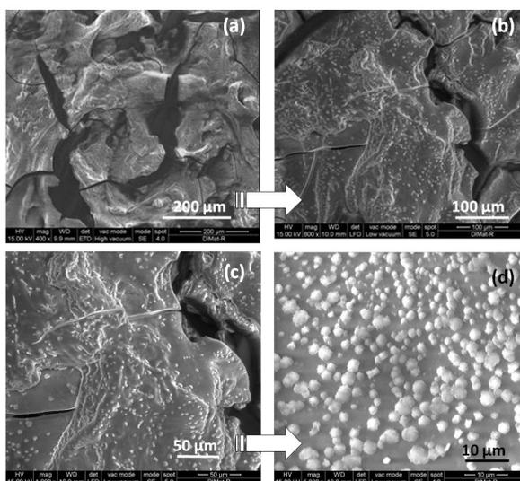
**Figure 5.** SEM micrographs for the Ly crystallization phenomena using 0.4 M PyO as crystallization agent in 0.1 M NaAc stock solution with different magnifications: (a) micrograph of a sample with a scale bar = 200 μm; (b) zoom of the first image, scale bar = 100 μm; (c) zoom of the second image, scale bar = 50 μm; (d) visualisation of Ly microspheres, scale bar = 10 μm.
