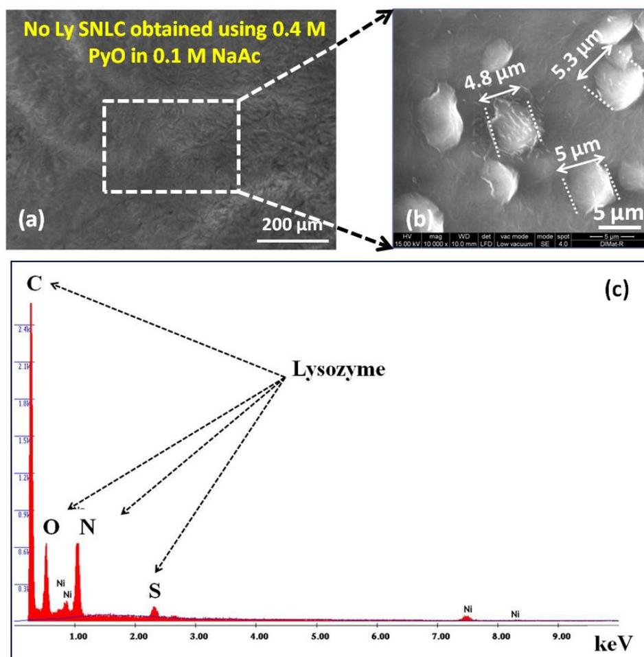
**Figure 6.** SEM micrographs and EDX analysis of the Ly crystallization phenomena using 0.4 M PyO as crystallization agent in 0.1 M NaAc stock solution.
