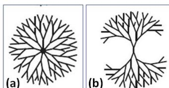
**Figure 1:** Schematic representation of spherulites type [Coleman & al., 1960 and Heijna & al., 2007]:
