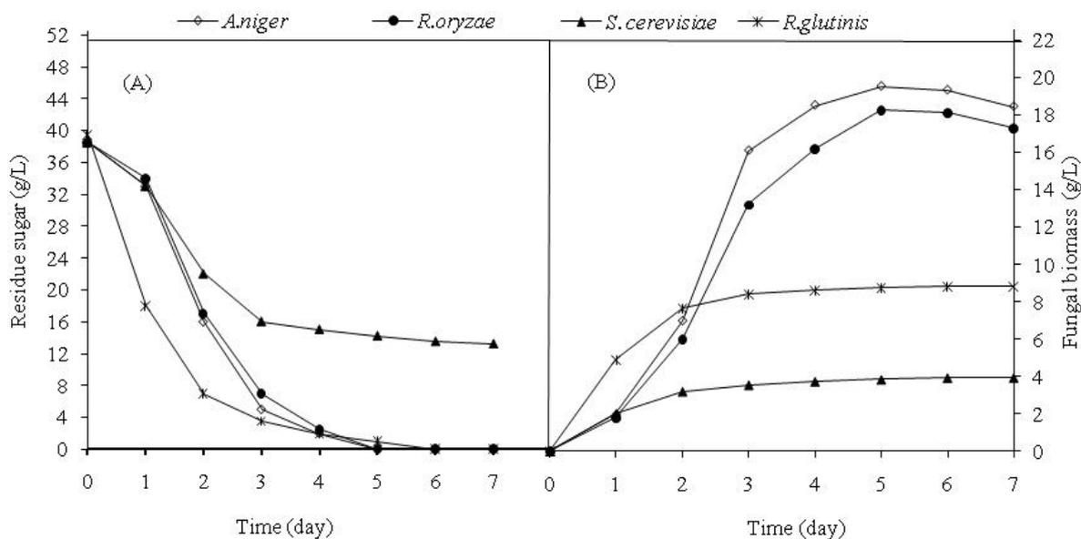
**Figure 3.** Time profiles of residue sugar (A) and fungal biomass (B) in the cultures of the test fungi cultivated in LKEM. Fermentation parameters: Loquat kernel extract (LKE) = 60 g/L, Peptone = 5 g/L, Temperature = 30°C, pH = 5.5 and Shaking speed = 200 rpm.
