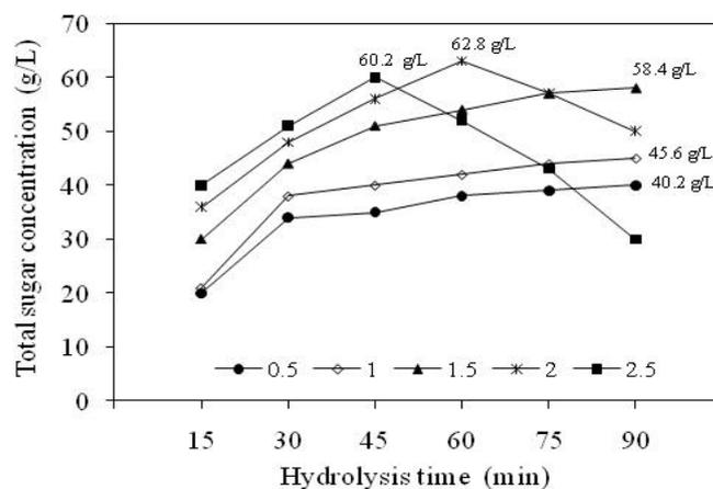
**Figure 1.** Time profile of total sugar contents in the hydrolysates prepared from 100 g loquat kernel flour (LKF) at the different H<sub>2</sub>SO<sub>4</sub> concentrations. Hydrolysis conditions in autoclave: 121°C and 1.2 atm. For each hydrolysis condition, maximal values are annotated.
