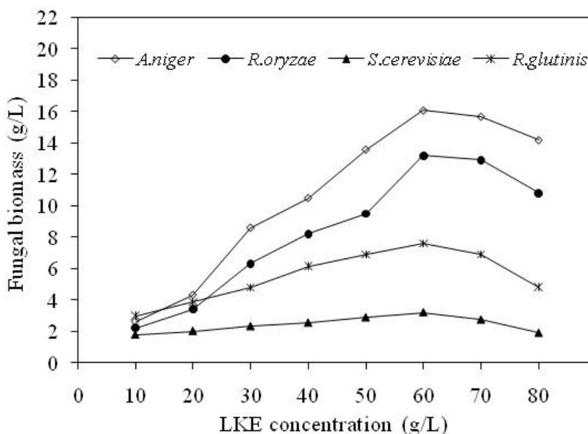
**Figure 2.** Biomass production by yeasts (for 2 days) and moulds (for 3 days) at the different loquat kernel extract (LKE) concentrations. Fermentation parameters: Peptone = 5 g/L, Cultivation temperature=30°C, pH = 5.5 and Shaking speed=200 rpm.
