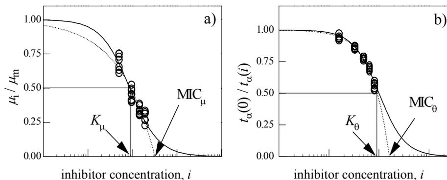
**Figure 4.** Calculation procedure involved in the determination of the quantitative parameters that characterize the growth inhibition of a microorganism by a certain inhibitor.
