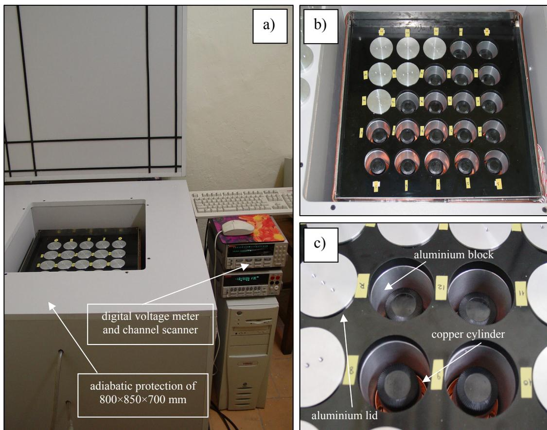
**Figure 1.** Isothermal calorimeter with 24 measurement units: a) general view; b) aluminium block in which the calorimetric cells are perforated; c) detail view of the calorimetric units containing vials with microbial cultures.
