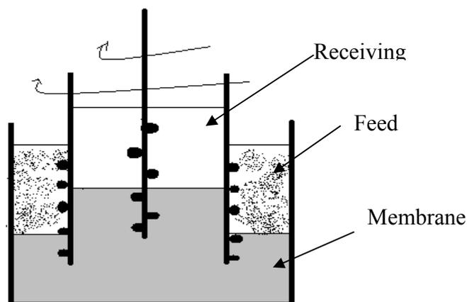
**Figure 1.** Experimental device used for the transport experiments.
