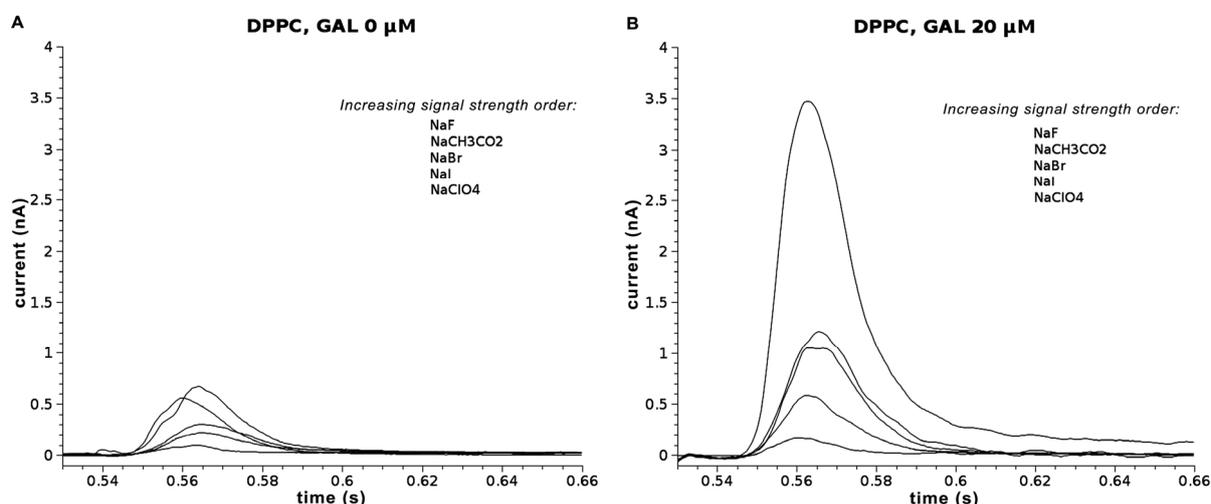
**Figure 2.** Electrical capacitive signals obtained after imposing concentration jumps of sodium salts of Hofmeister anions, without (A) and with (B) galantamine 20  $\mu\text{M}$ . The lipid used for membrane formation was diphytanoyl phosphatidylcholine (DPPC)
