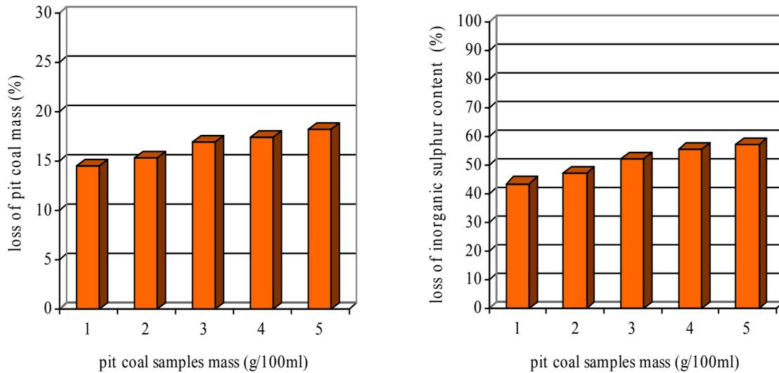
**Figure 5.** Variation of mass loss and inorganic sulphur content of pit coal from Mintia, in the presence of *Thiobacillus ferrooxidans* P<sub>9</sub> population, with the low tolerance to ferrous sulphate.
