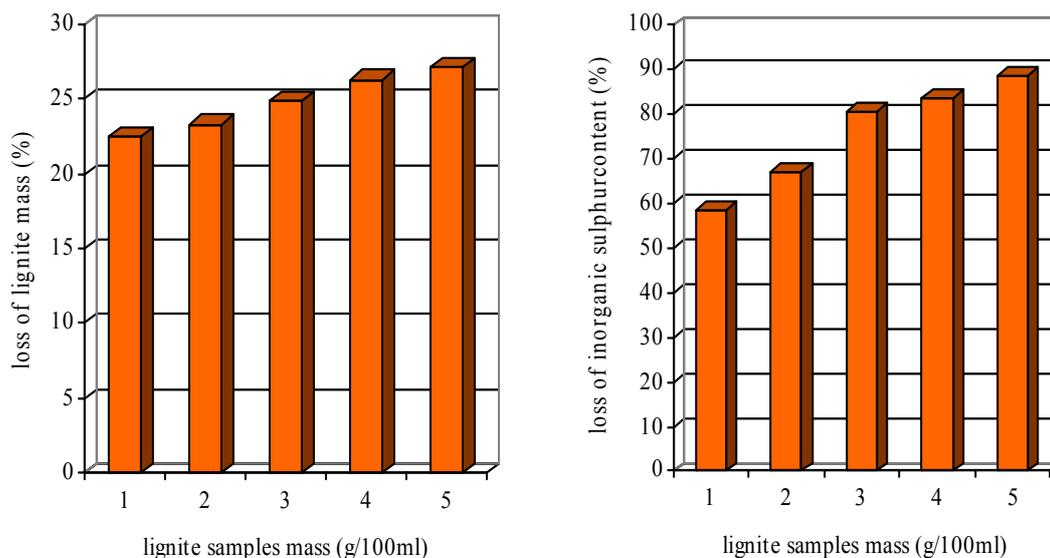
**Figure 8.** Variation of mass loss and of inorganic sulphur content of lignite from Halanga, in the presence of *Thiobacillus ferrooxidans* P<sub>7</sub> population, with the high tolerance to ferrous sulphate.
