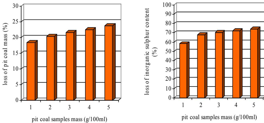
**Figure 6.** Variation of mass loss and of inorganic sulphur content of pit coal from Mintia, in the presence of *Thiobacillus ferrooxidans* P<sub>7</sub> population, with the high tolerance to ferrous sulphate
