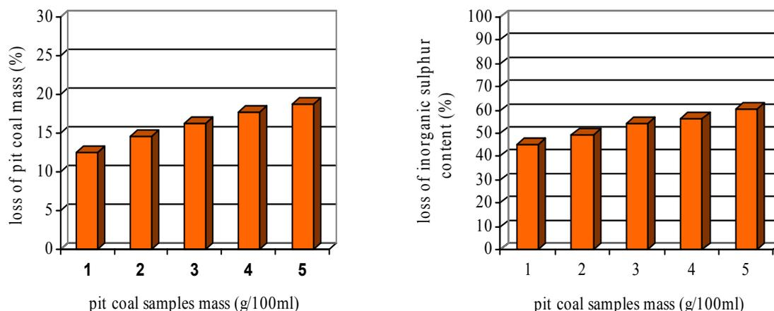
**Figure 4.** Variation of mass loss and of inorganic sulphur content of pit coal from Petrila, in the presence of *Thiobacillus ferrooxidans* P<sub>7</sub> population, with the high tolerance to ferrous sulphate.
