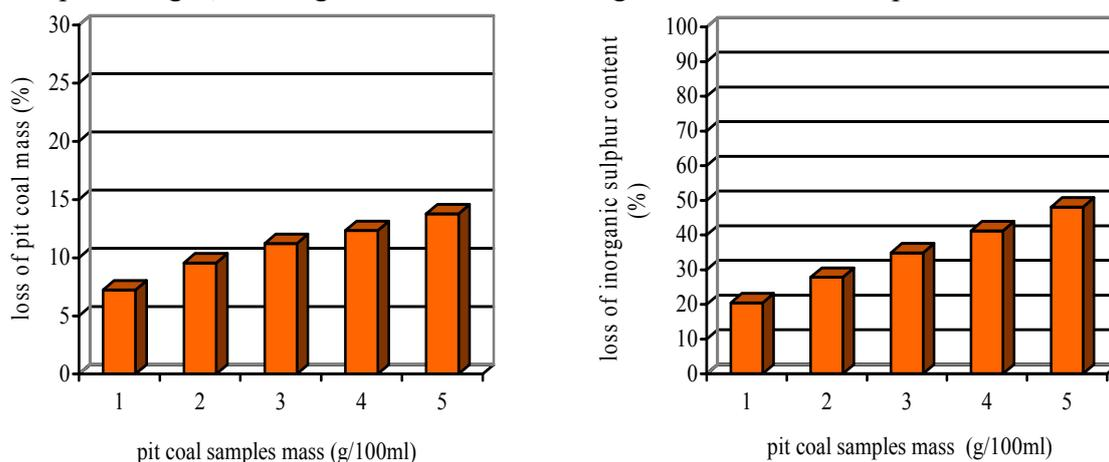
**Figure 3.** Variation of mass loss and inorganic sulphur content of pit coal from Petrila, in the presence of *Thiobacillus ferrooxidans* P<sub>9</sub> population, with the low tolerance to ferrous sulphate.
