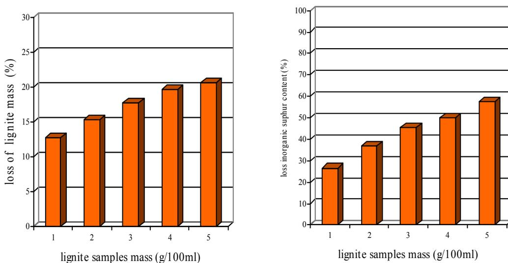
**Figure 7.** Variation of mass loss and of inorganic sulphur content of lignite from Halânga, in the presence of *Thiobacillus ferrooxidans* P<sub>9</sub> population, with the low tolerance to ferrous sulphate.
