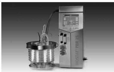
Fig. 7. Photobioreactor PBR 25 S for microalgae culture
