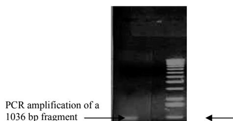
**Fig. 5.** F3 PCR. The distal primers F1FOR and F2REV initiated the fusion PCR of the gene-flanking genomic DNA sequences as a continuous fragment containing an *SmaI* cleavage site.
